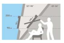
Top-operated centre-pivot roof windows make it possible to place furniture directly below the window without obstructing operation of the window.
